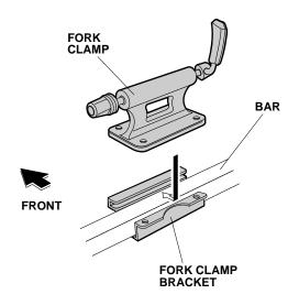
6. Using the torx wrench provided, secure the fork clamp to the fork clamp bracket with two bolts and two 6 mm washers.
