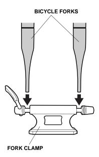
9. Lift the lever from the mid position to the closed lock position. While holding the lever on the fork clamp, turn the knob to put tension on the bicycle forks.
