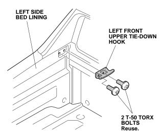
Reinstall the left front upper tie-down hook with the mounting bracket and two T-50 torx bolts. Torque the T-50 torx bolts to: 18.6 ~ 24.5 N·m (13.7 ~ 18.1 lbf·ft). Install in the following order (1 → 2).
